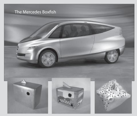
Mercedes Benz has unveiled a flashy concept car [top] modeled after the surprisingly aerodynamic boxfish [above right]. The car uses about 20% less fuel than other vehicles its size, the company claims. And, like the fish it's named for, it is lightweight but rigid and strong in key places. [Ed. note: The other two images – artists' interpretations of boxfish - have been placed here simply to confuse you.] Before saluting
